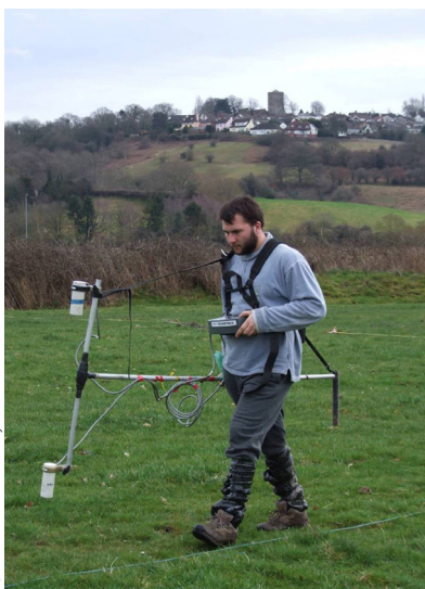
Figure 5 Geophysics: Sam Steele using a resistivitymeter
